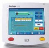
console. This allows the operator to easily handle the whole injection remotely. With user friendly interface the system gives operator easy to edit protocols and execution of injection, which synchronously display all operations in the local console as well as remote console.
